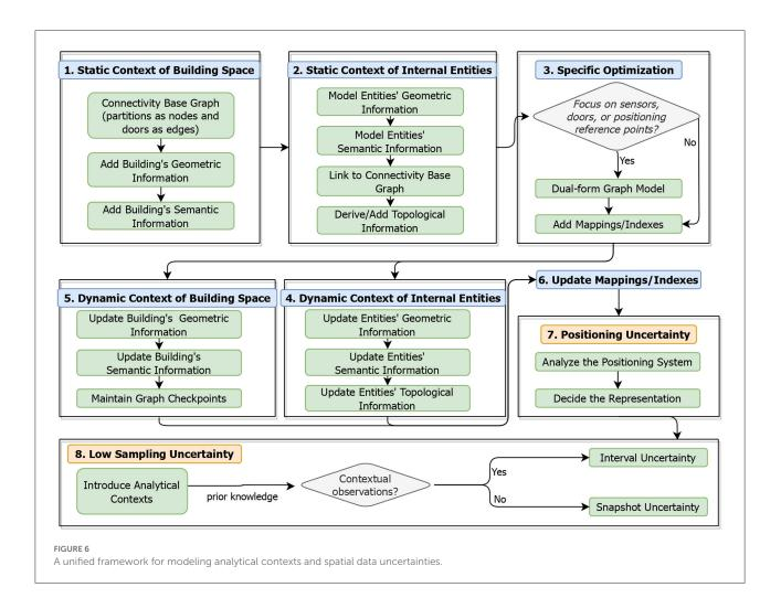
properties of each building element using object-oriented data models and link those data models to the components of the connectivity base graph (i.e., doors and partitions).
